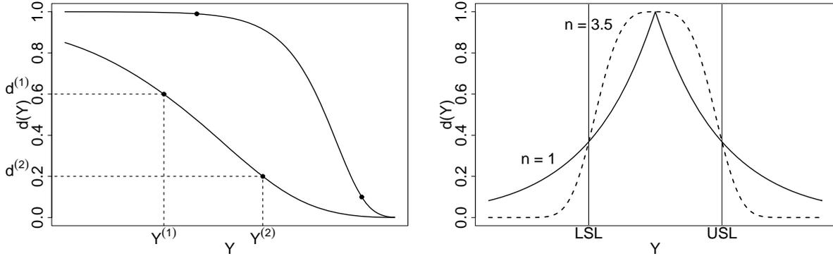
Figure 1: Harrington's one (left)- and two-sided Desirability Functions (right)
