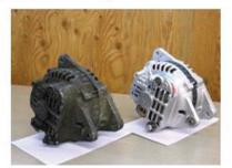
Used alternator (left) and remanufactured alternator (right)
