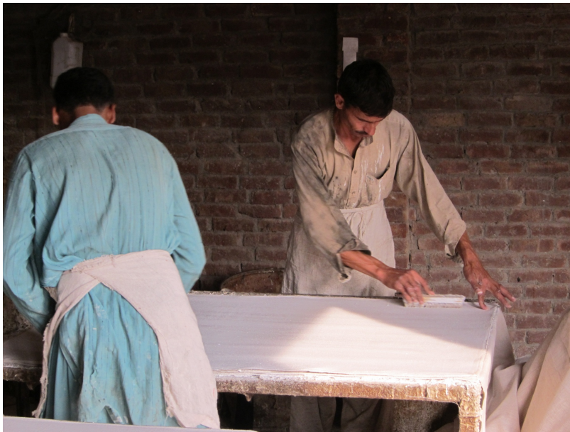
Figure 2: Making the Laminated Rexine Sheet (Step 1)
