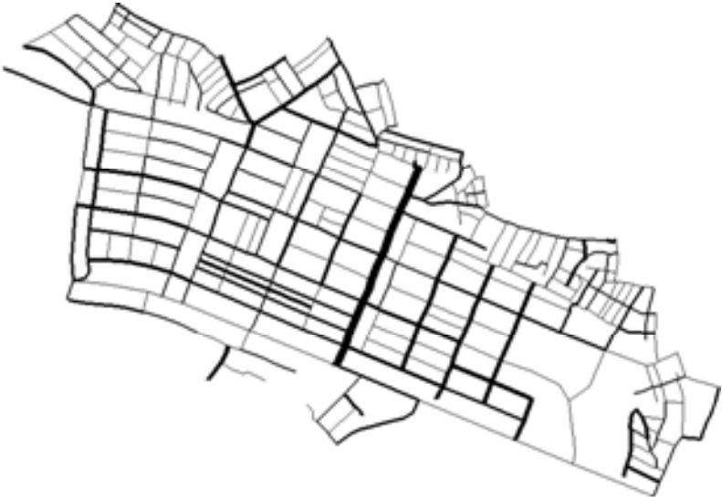
The thickness of the lines represent the length of BSUs (it is scaled at a factor of 0.01 in GRASS GIS).
