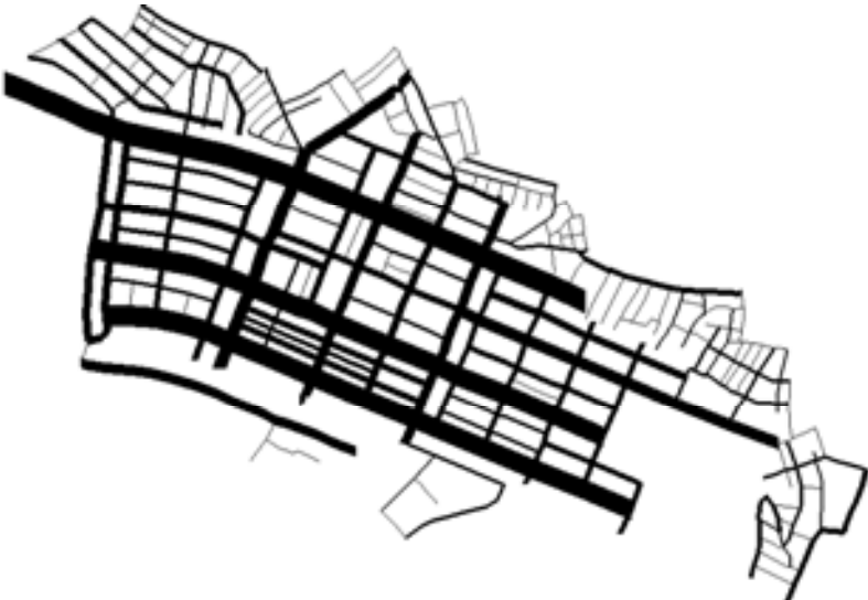
The thickness of the lines represent the length of streets (it is scaled at a factor of 0.01 in GRASS GIS).
