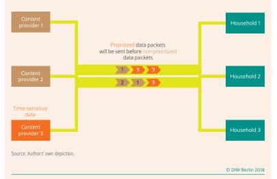
Time-sensitive data will be sent before non-prioritized data to ensure a smooth performance of time-sensitive applications. The transmission of non-prioritized data is delayed.
