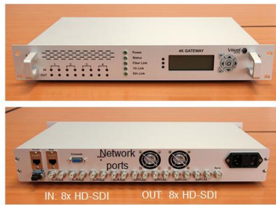
Figure7 MVTP-4K Box Enabling Multiple Video Transmissions
