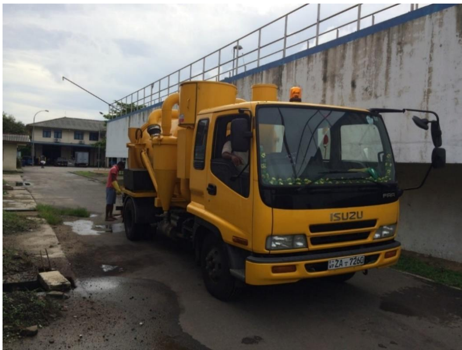
Figure 5: Delivering the fecal sludge to the wastewater treatment plant (Sri Lanka, 2017)
