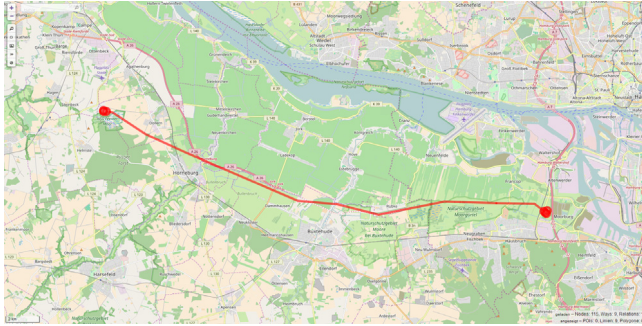
Fig. 3. Example of a power relation in OSM: relation with OSM-ID = 1188848 is composed of two substations (represented by square-like closed ways in red) and seven transmission lines (represented by the linear features in red colour). Credits: ©OpenStreetMap contributors, overpass-turbo.eu. (For interpretation of the references to colour in this figure legend, the reader is referred to the web version of this article.)
