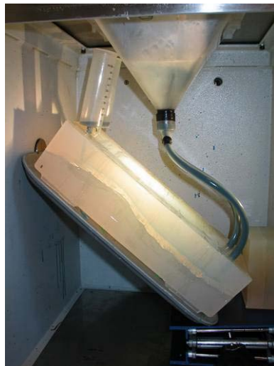
Figure 3. "Silicone mould, placed in vacuum chamber, after pouring with resin".
