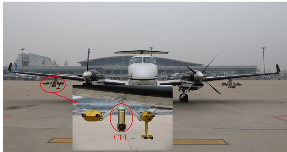
Figure 1. Photograph of the Cloud Particle Imager (CPI) under the aircraft wing at the Hebei, China.
