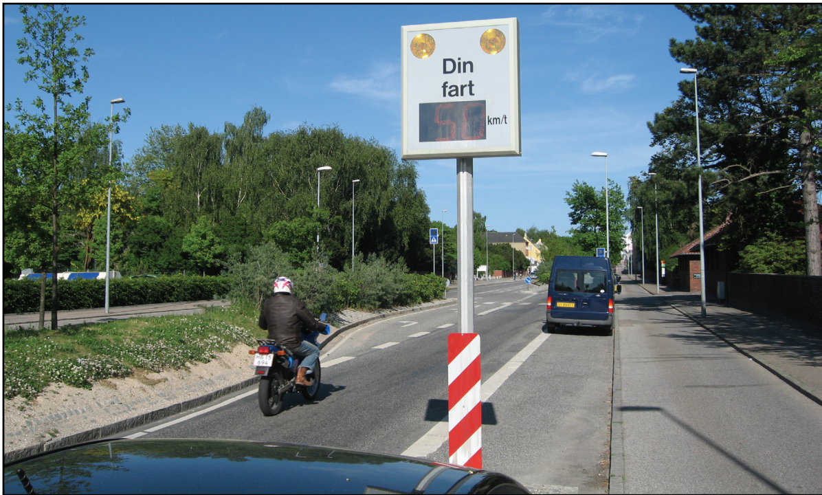
Figure 4: The external speedometer sign shows the speed (50 km/h) of the passing motor cyclist. He is able to see this when approaching the sign. The two yellow circular lights above the actual speed indicator will flash, if the motorist is exceeding the speed limit.
