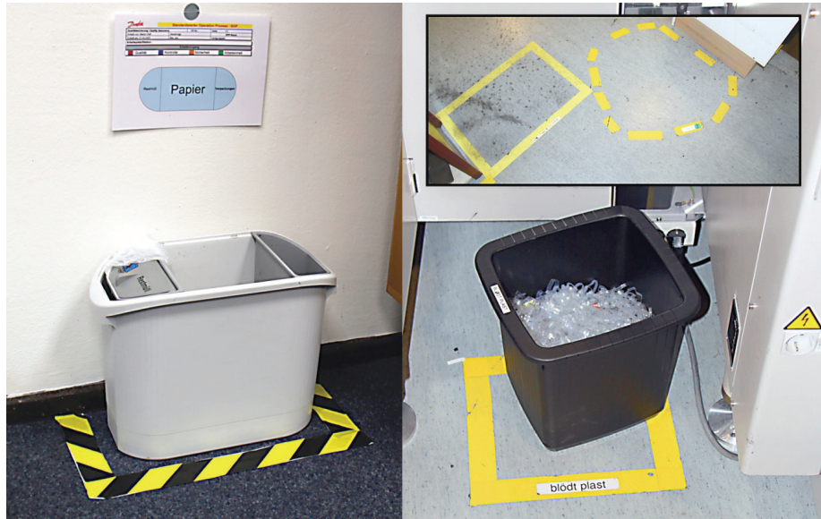
Figure 11: The concept of marking the proper place of a wastebasket.
