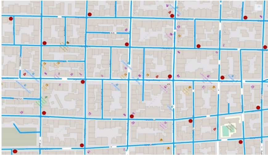
Figure 1. Scorched earth sample of trenching (blue lines) and FTTH cabinets (red points) in dense urban area in Greece
