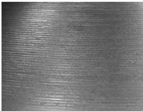
Fig. 7a. Rills caused by roller tool indentations
