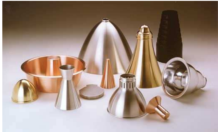
Fig. 2. Typical workpieces of shear forming, see Ott [1]
