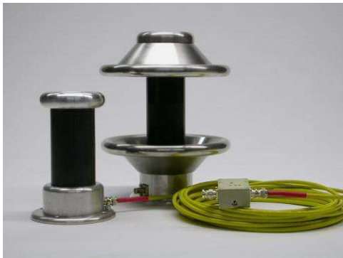
Fig. 3. Examples of high voltage dividers
