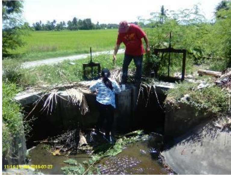
Photo 21. Water quality measurement in a Lateral (Marbel #1 RIS).
