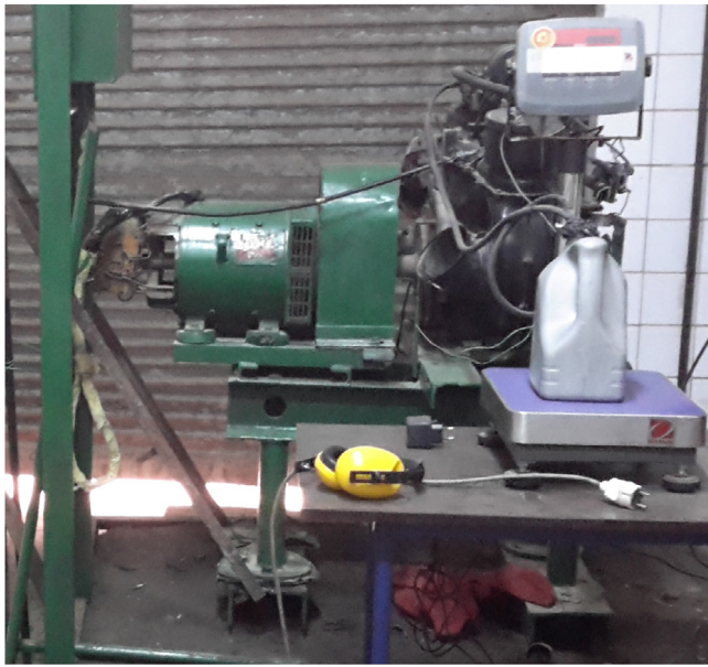
Fig. 1. The test room (engine and dynamometer) connected to the gas analyzer.
