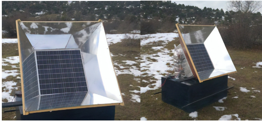
Fig. 3. Winter application of the concentrated photovoltaic panel/collector system, photo.
