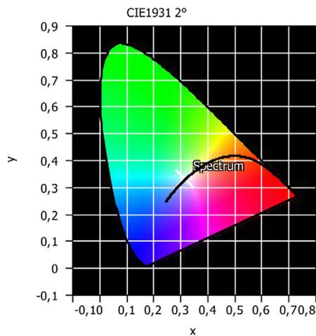
Fig. 16. Chromaticity coordinates for the LED lamp.
