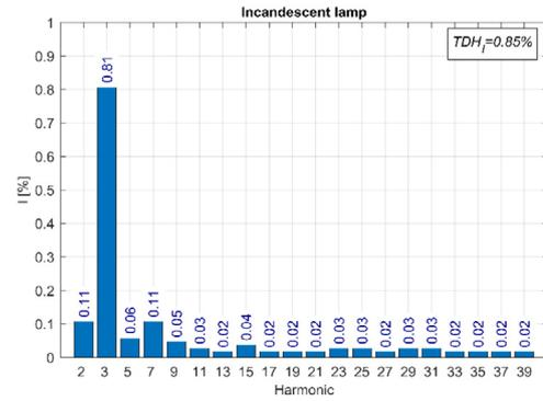
**Fig. 19.** Harmonic content of the halogen incandescent lamp.
