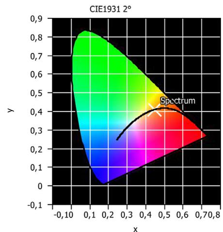
**Fig. 12.** Chromaticity coordinates for the halogen incandescent lamp.
