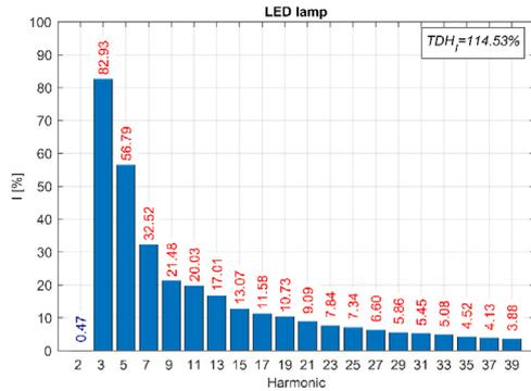
**Fig. 23.** Harmonic content for the LED lamp.
