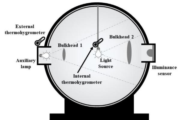
**Fig. 10.** Schematic of an integrating sphere of Ulbricht.
