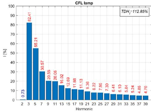
**Fig. 21.** Harmonic content for the halogen CFL lamp.
