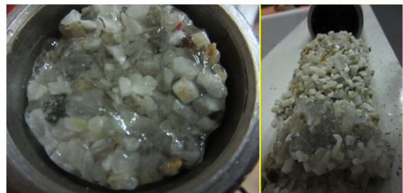
Fig. 6. Screening out of HPAM/chromium acetate gel within the first section of 6 Darcy marble pack. Length of the model – 8.6 cm, diameter – 4.3 cm.
