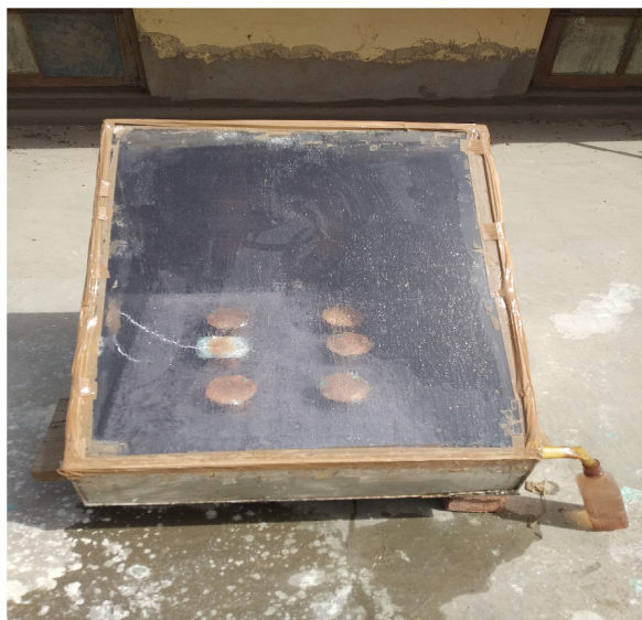
Fig. 2. Pictorial view of the experimental setup for solar still coupled with PCM stored in copper cylinder.
