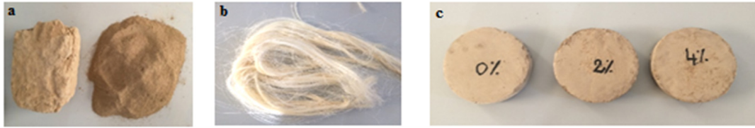
Fig. 2. (a) The raw clay material; (b) The sisal fibers; (c) the characterized samples.
