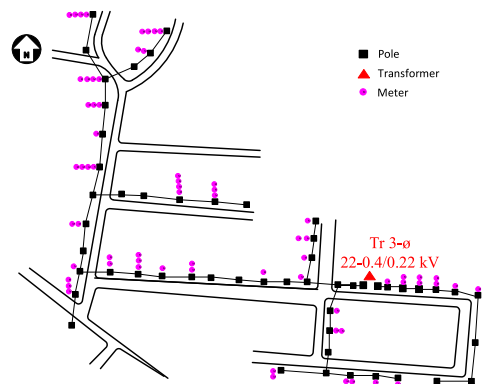
Fig. 2. Low voltage distribution system of the Provincial Electricity Authority in Chiang Mai which installed transformer 100 kVA.
