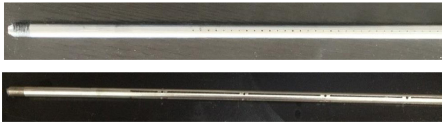
Fig. 5. Model of perforation well and slotted liner.
