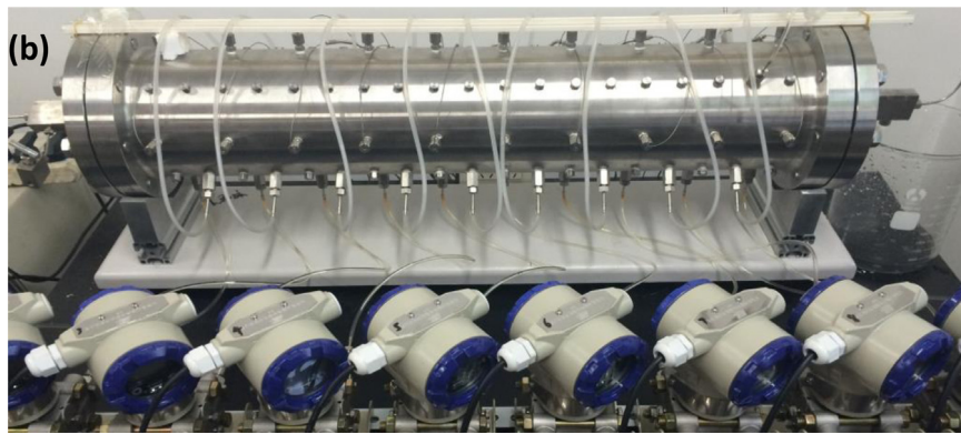
Fig. 4. The cylindrical horizontal wellbore model used in this study.
