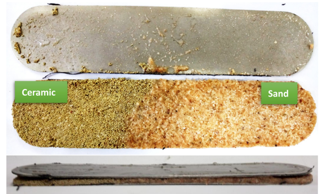
Fig. 4. Morphology of different proppants after the fracture conductivity test (Left-hand side represents the outlet and right-hand side represents the inlet, ceramic to sand ratio is 4:6 in this case).
