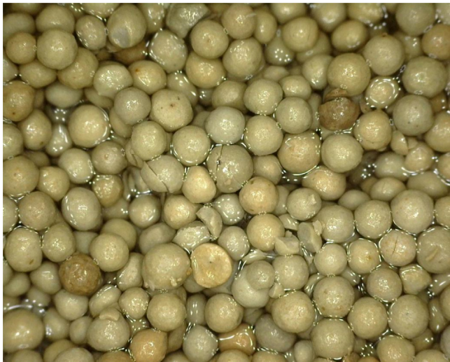
Fig. 6. Crushing of ceramic proppants near the outlet after conductivity test (ratio of ceramic proppants to sands is 4:6 in this case).
