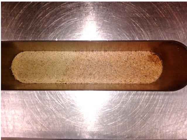
Fig. 3. Morphology of different proppants before the fracture conductivity test (Left-hand side represents the outlet and right-hand side represents inlet, ceramic to sand ratio is 4:6 in this case).
