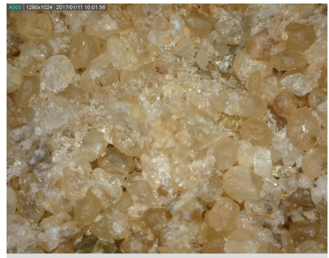
Fig. 5. Crushing of sands near the inlet after conductivity test (ratio of ceramic proppants to sands is 4:6 in this case).
