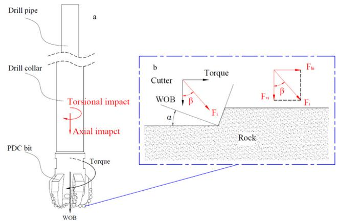
Fig. 2. Schematic of an analysis model with a sharp cutter: (a) a drilling model with compound axial and torsional impact loads; (b) the cutting model with an applied impact load ( $F_i$ ). In the model,  $F_{vi}$  is the vertical impact load,  $F_{hi}$  is the horizontal impact load,  $\beta$  is the impact angle, and  $\alpha$  is the rake angle of the cutter.
