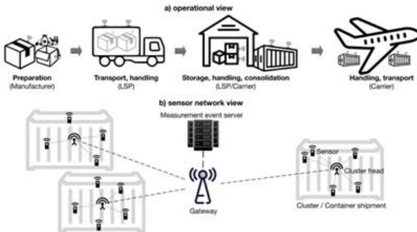
Figure 3: Operational and sensor network views of a cold pharmaceutical air SC (Konovalenko, Ludwig and Leopold, 2021)
