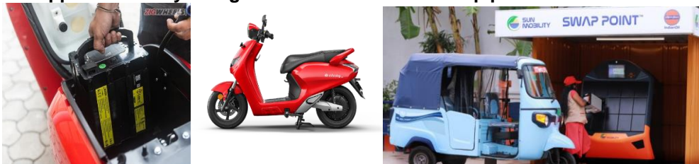
Figure 8: Illustration of how the depleted battery can be manually removed from an E2W or E3W and swapped for a fully charged one at a dedicated swap point
