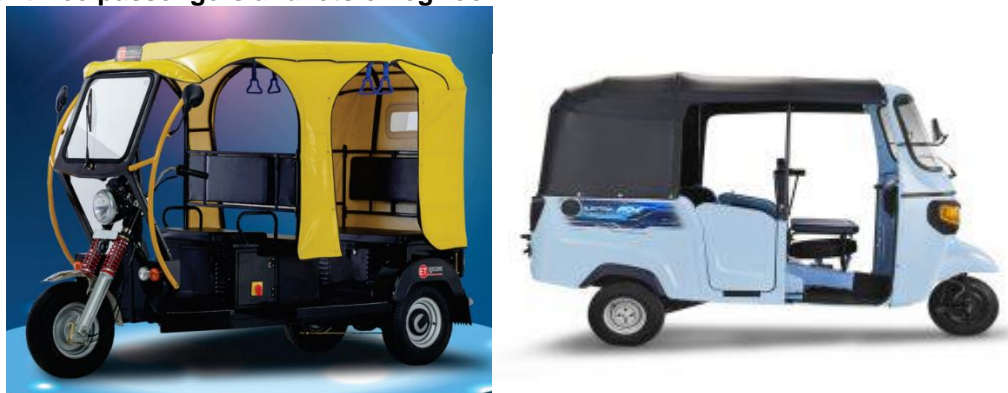
Figure 4: E3Ws for passengers. Left: two rear rows of seats facing each other. Right: one row of seats for three passengers and lots of leg room
