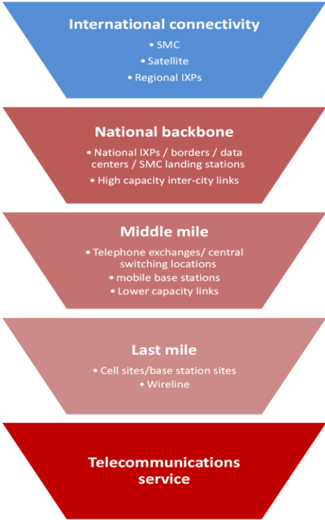
Figure 1. Infrastructures and international telecommunications access value chain
