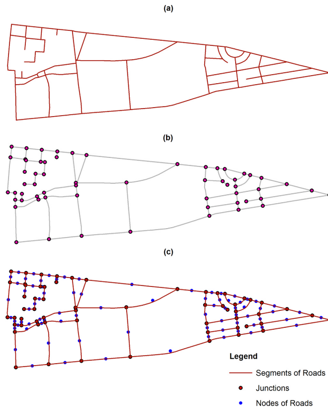
Fig. 2. Different ways of representing road transport network (a) the natural road network map (b) Primal Graph of Natural Road network (c) the Integrated Graph of Natural Road Network.
