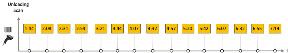
FIGURE A1 Time series of an unloading signal section for a JIS delivery
