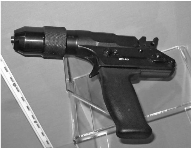
Figure 12.4 Pistol-style captive bolt stunner that uses a blank cartridge to propel the bolt. To insure maximum effectiveness, this tool requires three things: 1) careful cleaning and maintenance every day; 2) dry cartridges; 3) the correct cartridge size for the type of animal (photo credit: Temple Grandin).
