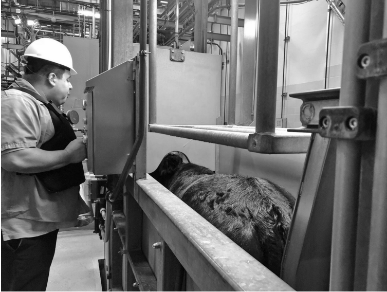
Figure 12.3 Single cattle stun box with a headholder to hold the head still for captive bolt stunning. This box must have a non-slip floor to prevent agitated behaviour due to slipping (photo credit: Temple Grandin).
