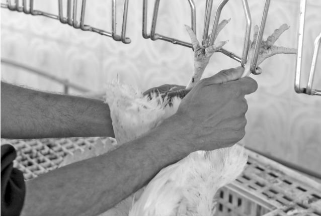
Figure 12.7 Shackling of live poultry to position them for water bath electrical stunning. The live birds are then moved by the conveyor to the water bath electrical stunner (photo credit: Daniel Schneider).
