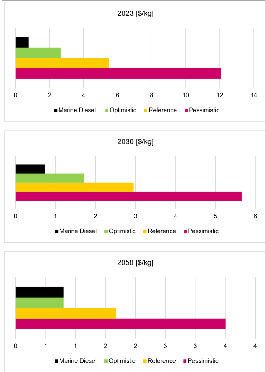
Figure 7: Cost comparison of e-diesel production costs in Chile, Patagonia with conventional marine diesel
