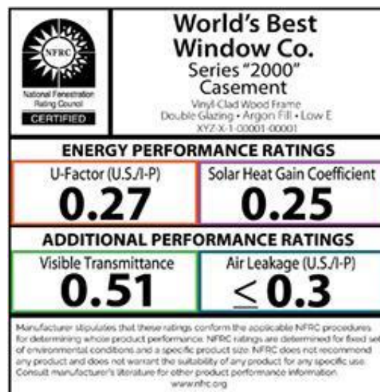
Figure 7: Window Label from the National Fenestration Rating Council in the United States
