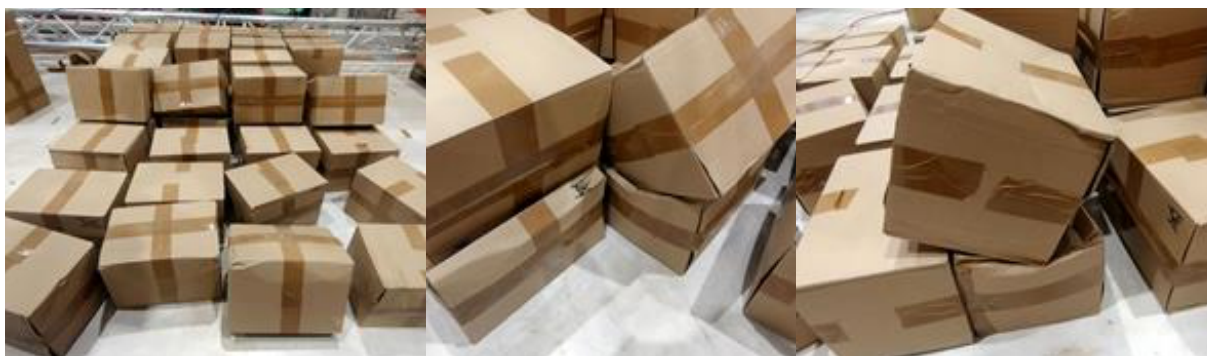
Figure 10: A collapsed wall of parcels (left) and incurred damage on parcels in detail (middle and right)
