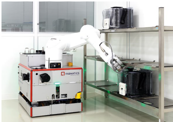
Figure 2: Multiple-load AGV equipped with a robot arm handling at a shelf in a semiconductor production facility (reference: www.fabmatix.com )
