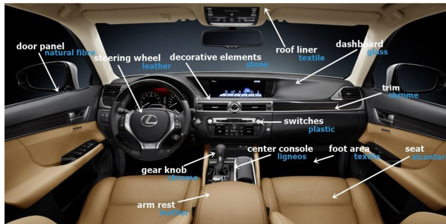
Fig. 8 Interior components with corresponding materials. Source: Barnes-Clay, 2012
