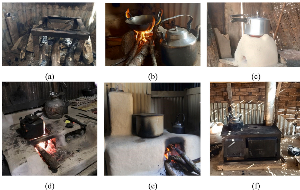
Fig. 3. Study stoves. (a) Traditional Open Fire (b) Three Stone (c) Mud Stove (d) Metal Frame Mud Stove (e) Mud Stove with chimney (f) RPN stove.
