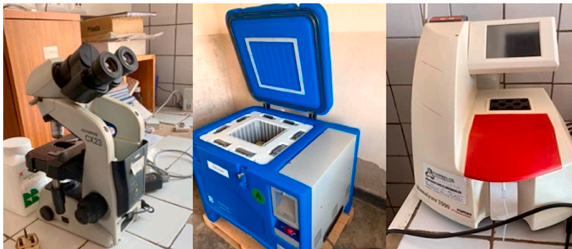
Fig. 7. Appliances powered by OffGridBox at health clinics in Rwanda. From left to right: Microscope, Vaccine Refrigerator, and Chemical Analyzer.
