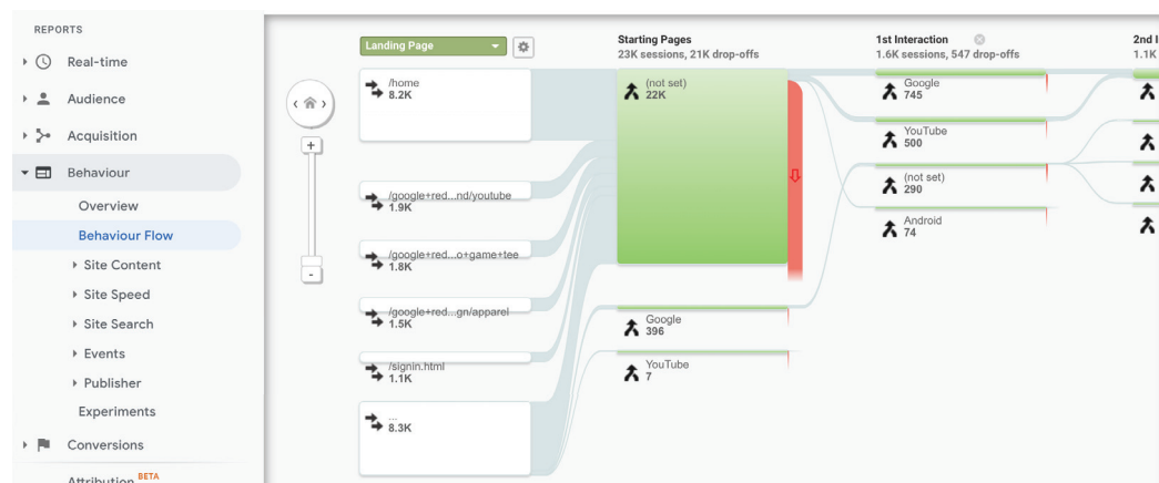
Figure 2. Example of the “Behavior flow” report in Google Analytics. It shows the sequence of most visited pages, from left to right. The thick red lines indicate traffic drop-offs. Each column corresponds to a web page or event. Therefore, this type of visualization does not show all the navigation in a single view but continues to the right, according to the number of pages or events.
