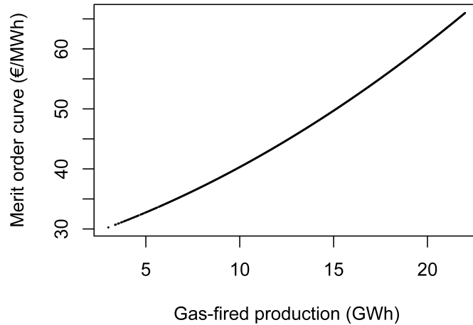
Figure 6: Estimated gas-fired merit order curve based on average gas and carbon emissions prices. Coefficients from the quadratic regression model estimated on the series for unsold electricity.
