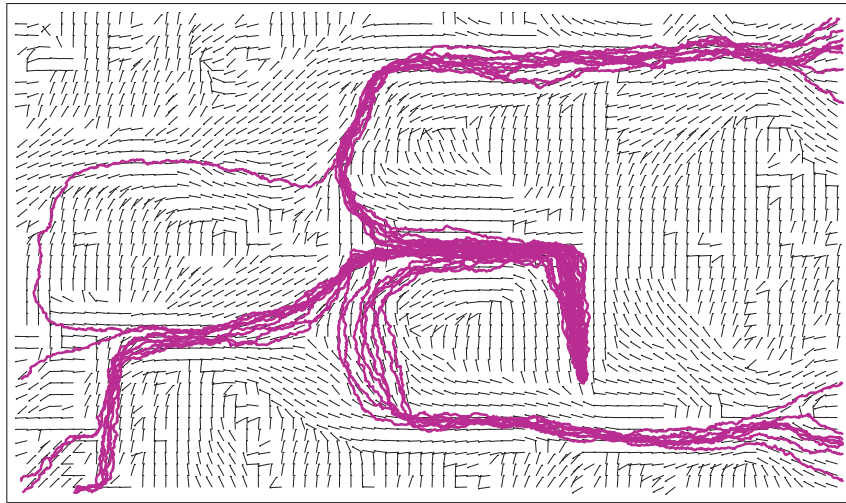
Figure 4: A bundle of 25 random tracks generated by Algorithm T1 with parameters \Delta t = 0.1 , \sigma = 0.2 . The vector field and the starting point for tracking are the same in Figures 3-6.
