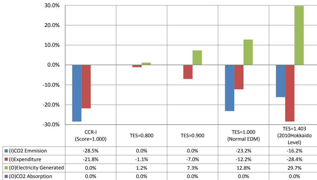
Figure 9 Efficiency improvement projection results based on the TS-EDM (Hokkaido 2011)
